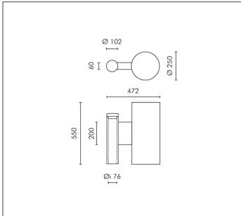
HIT-DE 150W CLEAR Rx7s 13250lm Rated luminaire luminous flux: 7817lm
