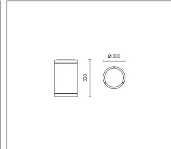
HIT-CRI 70W CLEAR G12 6600lm Rated luminaire luminous flux: 3168lm
