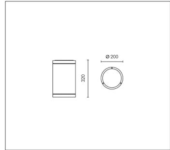
TC-TEL 26/32/42W Gx24q-4 3200lm Rated luminaire luminous flux: 1312lm
