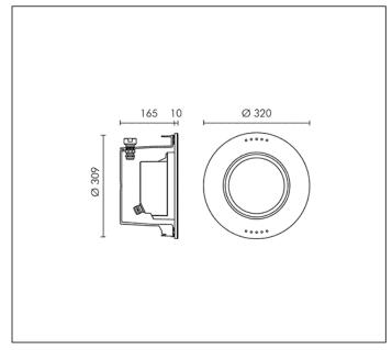
12 MODULES LED RGBW 24V PWM Rated luminaire luminous flux: 430lm Rated input power: 31W
