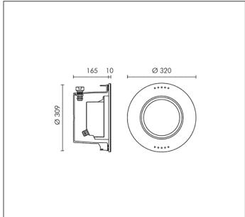
12 MODULES LED RGBW 24V PWM Rated luminaire luminous flux: 430lm
