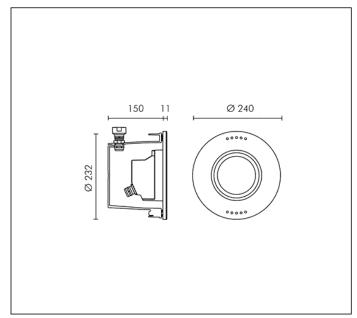
5 MODULES LED RGBW 24V PWM Rated luminaire luminous flux: 206lm
