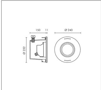
6 MODULES LED 6000K 24V 1670lm CRI 70 Rated luminaire luminous flux: 891lm
