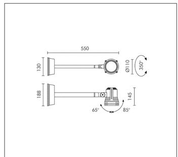
QT12 35W ES GY6,35 12V 900lm Rated luminaire luminous flux: 549lm
