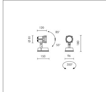
HIT-TC CRI 20W G8,5 1700lm Rated luminaire luminous flux: 765lm
