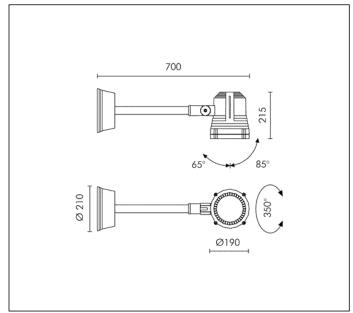
HIT-CRI 70W CLEAR G12 6600lm Rated luminaire luminous flux: 3432lm
