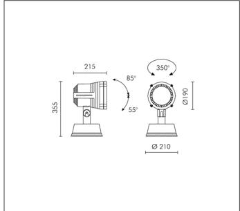
HIT-CRI 70W CLEAR G12 6600lm Rated luminaire luminous flux: 3432lm
