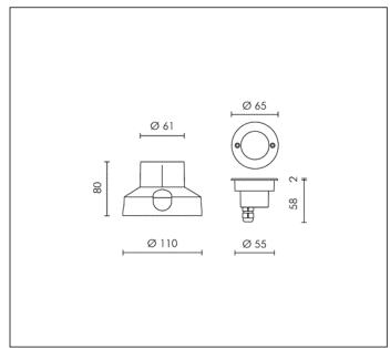
MODULES LED 6000K 24V c.c. CRI 75 Rated luminaire luminous flux: 40lm
