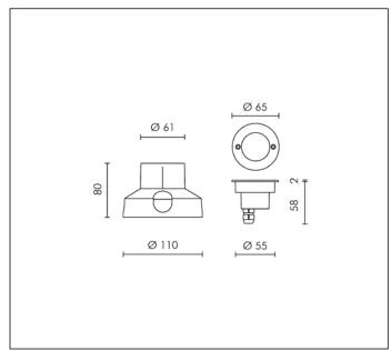
MODULES LED RGB 24V PWM Rated luminaire luminous flux: 40lm
