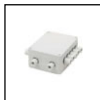
S.3401 BOX IP 55 WITH ELECTRONIC POWER SUPPLY 10W 24V D.C. (Electronic power supply included) Dimensions: 230 x 210 x 80 mm. Cable IN: 2 with cable glands PG11 Cable OUT: 6 with cable glands PG11 IP55 CLASS II The Total power of all connected luminaires may not be higher than the power of the driver.
