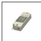
S.3400 ELECTRONIC POWER SUPPLY 10W 24V D.C. IP20 In: 240V Alternate Current Out: 24V Direct Current. The Total power of all connected luminaires may not be higher than the power of the driver. Dimensions: 120 x 35 x 20 mm.
