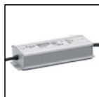
S.3407 REMOTE POWER SUPPLY 100W IP66 for monochromatic LED 100W 240V/24V DC. IP66 The Total power of all connected luminaires may not be higher than the power of the driver. Dimensions 210mm x70mm x40mm
