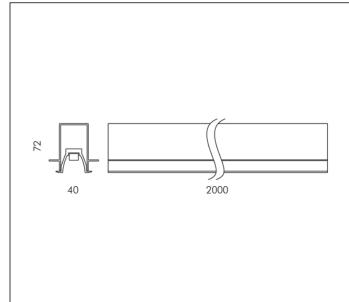
MODULES LED 3000K 24V 1600lm CRI 90 Rated luminaire luminous flux: 1600lm
