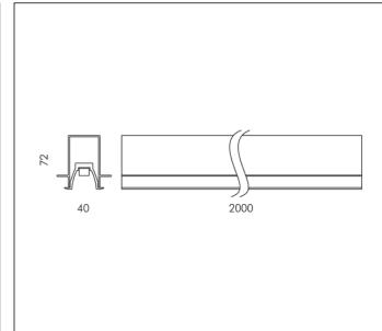
MODULES LED 4000K 24V 1600lm CRI 90 Rated luminaire luminous flux: 1600lm
