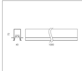
MODULES LED 3000K 24V 800lm CRI 90 Rated luminaire luminous flux: 800lm Rated input power: 11.5W Luminaire efficacy: 70lm/W
