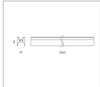
MODULES LED 3000K 24V 4000lm CRI 90 Rated luminaire luminous flux: 4000lm Rated input power: 57.5W
