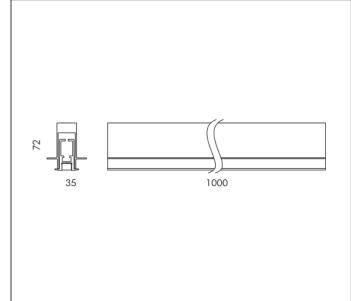
MODULES LED 3000K 24V 800lm CRI 90 Rated luminaire luminous flux: 800lm Rated input power: 11.5W
