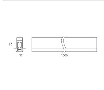
MODULES LED 4000K 24V 800lm CRI 90 Rated luminaire luminous flux: 800lm Rated input power: 11.5W Luminaire efficacy: 70lm/W
