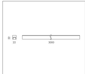
MODULES LED 4000K 24V 2400lm CRI 90 Rated luminaire luminous flux: 2400lm
