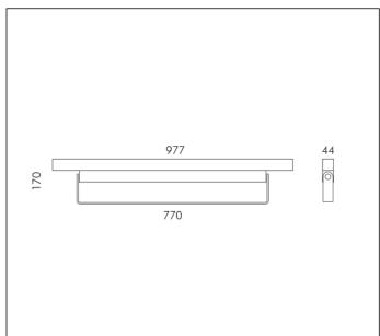
MODULES LED 3000K 230V 7920lm CRI 90 Rated luminaire luminous flux: 5500lm
