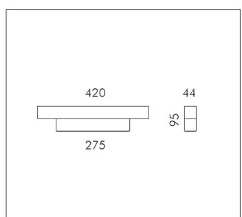
MODULES LED 4000K 230V 2960lm CRI 80 Rated luminaire luminous flux: 1751lm
