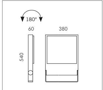
MODULES LED 4000K 230V 20457Im CRI 80 Rated luminaire luminous flux: 14195Im Rated input power: 147W
