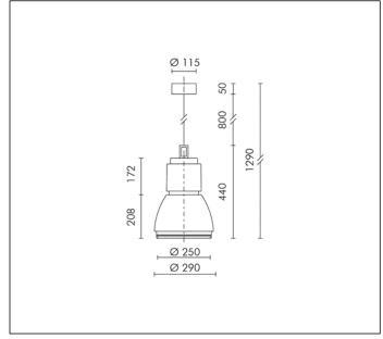
TC-TEL 26/32/42W Gx24q-4 3200lm Rated luminaire luminous flux: 1856lm
