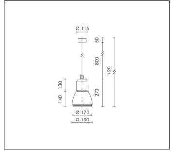
HIT-TC CRI 35W CLEAR G8,5 3300lm Rated luminaire luminous flux: 2343lm
