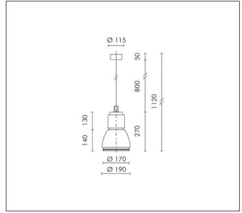
HIT-TC CRI 20W G8,5 1700lm Rated luminaire luminous flux: 1173lm
