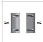
S.1013 FLANGE FOR POLE INSTALLATION Ø 120mm Flange in die-cast aluminium suitable only for Ø 120 mm poles. The flange can be used for maximum 2 projectors, one for each side.
