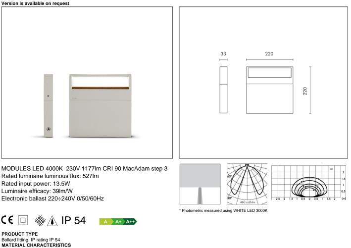
Aluminium die cast housing in EN AB-47100 (low copper content) with high resistance against corrosion. Extruded EN AW-6060 aluminium structure (bollard version) with high corrosion resistance. Oiled TEAK wood finish 8mm thick. Stone wash surface treatment prior to painting process. A4 grade Stainless Steel screws with 2,5-3% molybdenum content which increases the resistance against corrosion. Silicone gaskets. Painting Process : 3 Step Process
