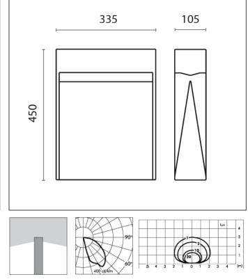
\* Photometric measured using WHITE LED 3000K
