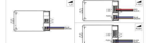
For more detailed information check wiring diagrams in catalogue or technical downloads at www.supermodular.com.
