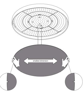
Be careful not to damage the LEDs when inserting the diffusor.
