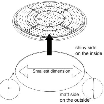
Be careful not to damage the LEDs when inserting the diffusor
