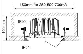
CAN BE USED WITH 130730XX Wink 115 flange 14204030 Recessed ring Ø146 Drivers: see driver matrix - latest version on website www.supermodular.com or check sales contact
