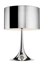
Table/desk lamp providing diffused light. Spun metal frame and diffuser, die-cast aluminum diffuser support arms and lampholder support, painted in the colors indicated below. White, injectionmolded polycarbonate diffuser supports. Sandblasted pressed glass upper diffuser screen. On the cable there is the electronic dimmer which allows the regulation of light brightness.
