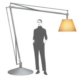
Floor lamp providing direct and diffused light. Acid-etched handblown pressed borosilicate glass internal diffuser. Plissé cloth external diffuser. Sand-cast, aluminum diffuser support. Gray painted assembly composed of tubular aluminum arms and tie rods, stainless steel springs, and die-cast aluminum joints. Sandcast aluminum base with gray painted spun aluminum cover. On the cable there is the electronic dimmer which allows the regulation of light brightness.
