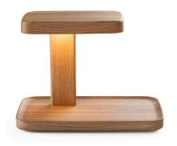
Table lamp with direct light. The shelf, stem and head are in American Oak or in basaltina stone. The diffuser is in double satinized methacrylate with silk-screen printing on the inside. The power cable is 2.5 metres long. The power supply is on a plug with interchangeable sockets.
