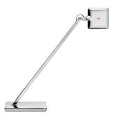
Table lamp providing direct light. Head in pressofused aluminium, diffuser in photo-engraved methacrylate with aluminate surround. Power pack on plug, base in pressofused zamak. Directionable head. ON/OFF switch with Soft Touch technology and light flow adjustment to 2 intensities (100% – 50% – 0%). Power pack on plug with interchangeable plugs.
