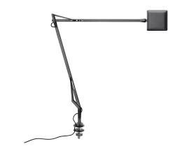
Adjustable table lamp providing direct light. Aluminium painted or chromed body, with die cast head, joints and forks, and extruded arms. Diffuser in photoengraved polycarbonate and aluminate on the perimeter. Edge Lighting technology light source. Optical switch sensor placed on the head that provide 3-step dimming function and color temperature adjustment at 2700K or 3200K. Power cord length 150 cm. Plug-in power supply with interchangeable plugs.
