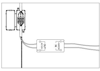
2. Connect the three power wires according to their colours. Brown is the live wire, blue is the neutral wire, green/yellow is the earth wire.
