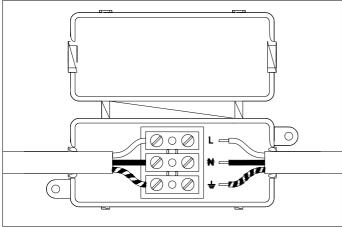
Connect the 3 power wires according to their colours. Brown is the live wire, blue is the neutral wire, green/yellow is the earth wire.
