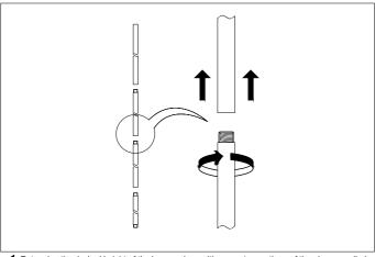
Determine the desired height of the lamp and use either one, two or three of the pipes supplied.
