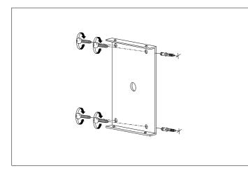
$\ensuremath{\textbf{1}}$  . Fix the wall plate to the wall by using wall mounting plugs and screws suitable to your wall type.
