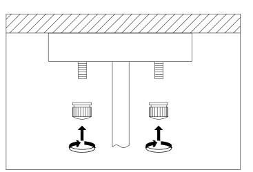
$\ensuremath{\textbf{4.}}$  Place the ceiling canopy over the ceiling plate and fix it securely with the four nuts.
