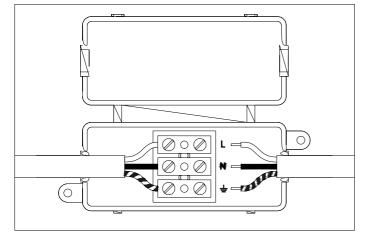
3. Connect the 3 power wires according to their colours. Brown is the live wire, blie is the neutral wire, green/yellow is the earth wire.
