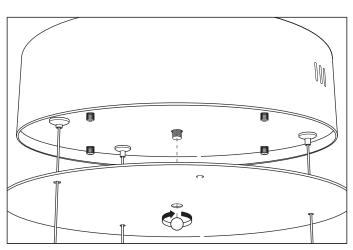
**6.** Place the ceiling plate over the canopy. Fix the ceiling canopy securely with the nut.
