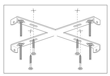
1. Fix the crossbar to the ceiling by using mounting plugs and screws suitable to your ceiling type. Place or hold the lamp in an elevated position in such a way that the wires can freely reach the ceiling junction box.
