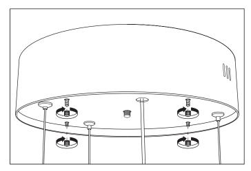
5. Place the ceiling canopy over the crossbar. Fix the ceiling canopy securely with the nuts.
