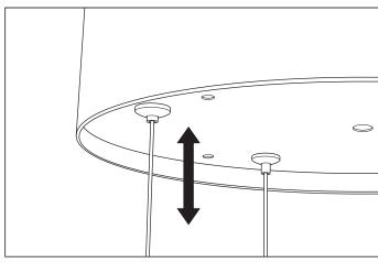
**3.** Adjust the height of the steel wires by pressing the wire lock on the ceiling canopy and pulling/pushing the wire through.
