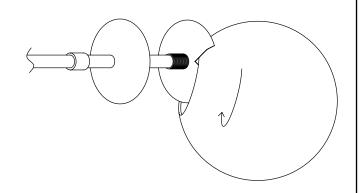
**3** Align the glass lampshade with the lamp holder. Fix the glass by tightening the nut.
