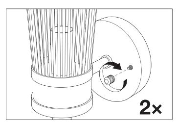
4. Fix the lamp securely with the knobs.
