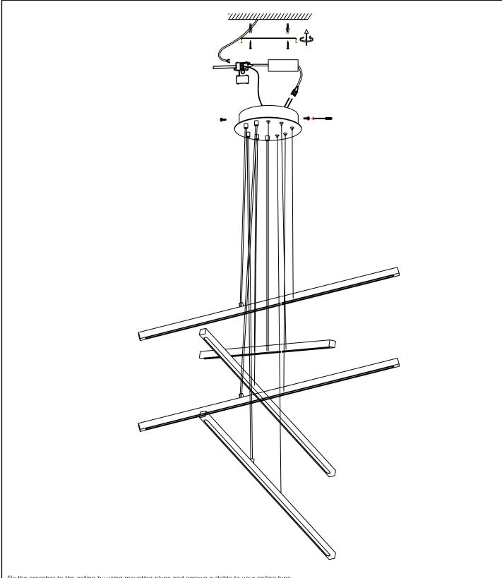
Fix the crossbar to the ceiling by using mounting plugs and screws suitable to your ceiling type.
