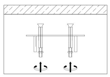
Fix the ceiling plate to the wall by using ceiling mounting plugs and screws suitable for your ceiling type.
