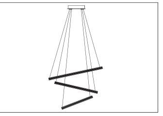
**2.** Determine the approximate desired height of the lamp and position of the rings and adjust the length of the steel wires by pressing the wire lock on the ceiling canopy and pulling/pushing the wire through. Adjust the height of the electric wires by pulling them through the wire nuts and fix each wire in the correct position with the screw on the side.
