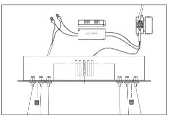
4. Place the canopy over the crossbar and fix it with the four nuts.
