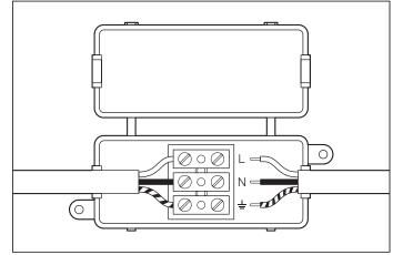
3. Connect the 3 wires according to their colours. Brown is the live wire, blue is the neutral wire, green/yellow is the earth wire.
