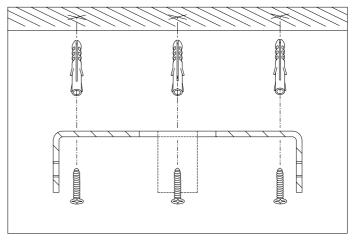
2. Fix the ceiling plate to the ceiling by using mounting plugs and screws suitable to your ceiling
