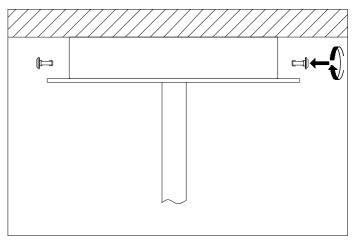
**4.** Place the ceiling canopy over the ceiling plate and fix it securely with the four nuts.
